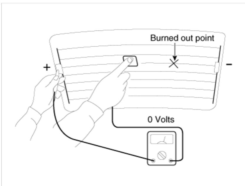
4. To check for open circuits, Slowly move the test lead toward the section where open circuits seem to exist. Try to find a point where the voltage turns to 0V. The point where the voltage has changed is the open-circuit point.
