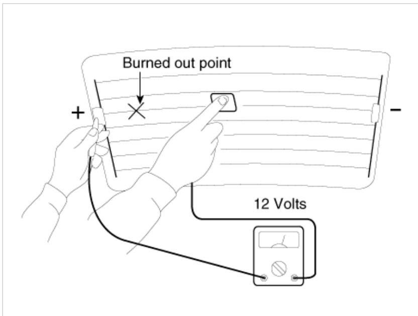
3. If a conductive line is burned out within the area between the central part and (-) terminal, the voltmeter will indicate 0V.
